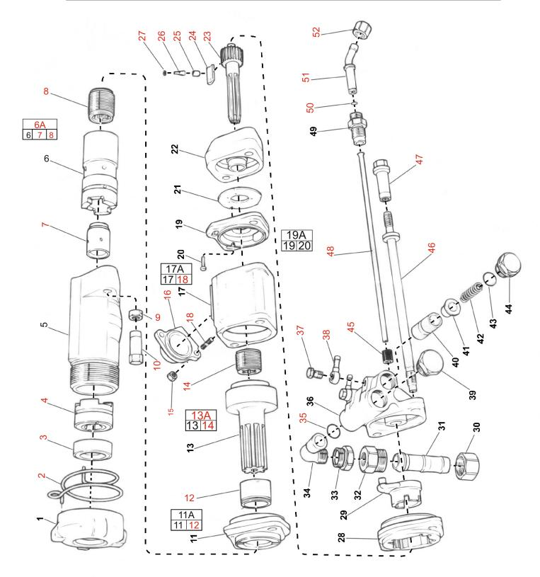
Note : Part number display in Red Colour are fast wearing parts and are recommended for stocking.
